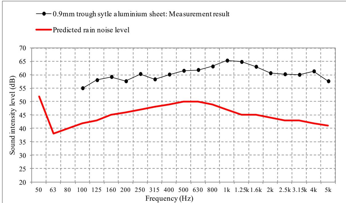
Figure 6 - Comparison of predicted and measured rain noise data (Trough style profile aluminum sheet)
