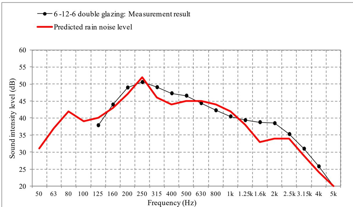
Figure 5 - Comparison of predicted and measured rain noise data (6-12-6 double glazing)
