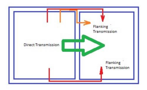
The picture above shows a few of the possible flanking paths (in red). With 2 rectangular boxes joined together on one face there are 12 possible flanking paths that will contribute
