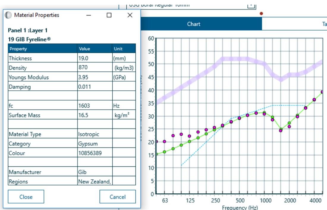
If you do not have any test data on the material then you need to know the density of the material, the Modulus of Elasticity and if possible the internal damping of the material (if damping is not known set it to 0.01). This data (density, E and damping) can now be entered into the materials editor.
