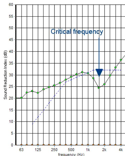
Above the critical frequency the TL increases at 12 dB/octave (doubling at frequency) so that as the frequency increases the TL can increase to above the mass law.
