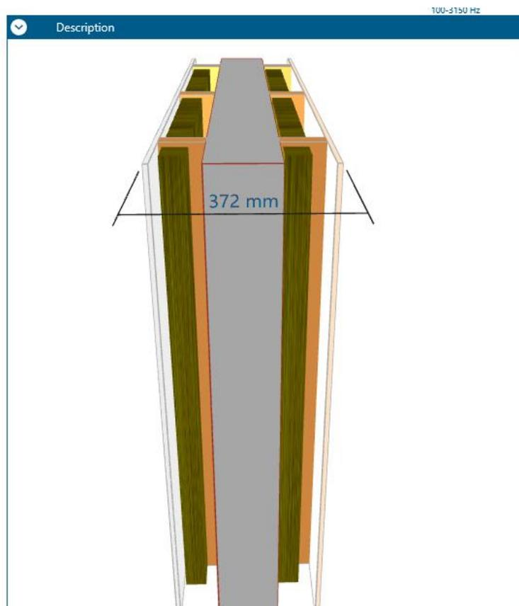
To predict triple panel constructions work your way across the various elements of the partition, entering or selecting the properties of each element (panel, frame etc) as you go.
