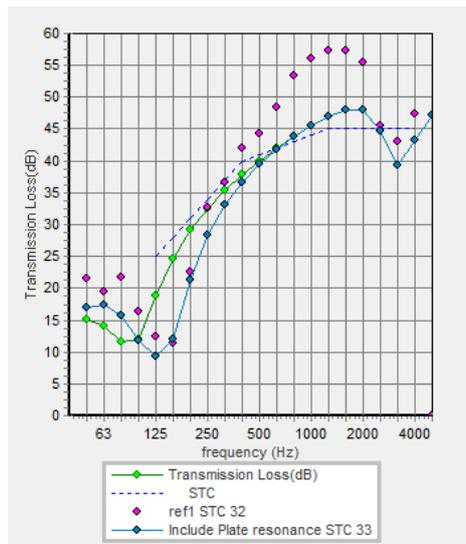
This effect is most important for small stud spacing's say (16" or 400mm), it is not so noticeable with stud spacing's of 24" (or 600mm).
