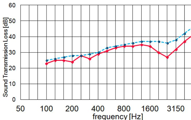
INSUL can model these as elastic core materials. Thus the user can experiment with different thicknesses of glass (as Side A and Side B) and different inter-layers (Core) to optimise the performance. There are a number of standard inter-layers such as DuPont's Butacite® that can be used from a drop down list in the materials editor.
