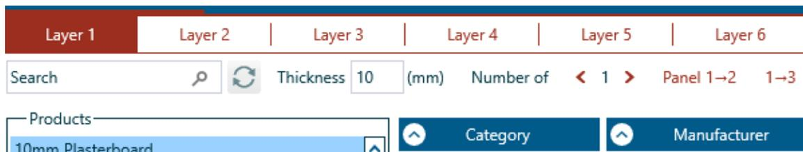
By using the inner and outer layer pages you can for instance have 3 layers of 16 mm plasterboard and 2 layers of 6 mm plywood.
