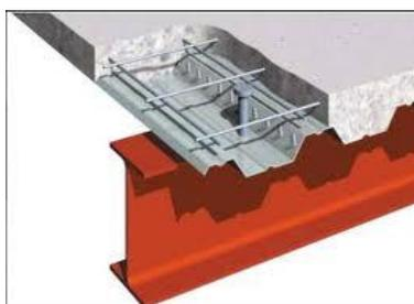
The different stiffnesses in the directions parallel and perpendicular to the steel profile give the floor different critical frequencies in each direction, that is the panel is orthotropic
