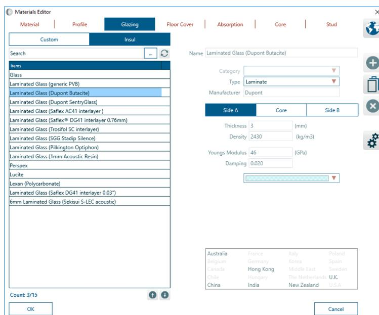
While the primary motivation of this development was laminated glass, this model could be used for other types of laminated materials including gypsum plasterboard with visco-elastic inter-layers.
