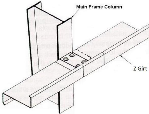
Z Girts are used in many countries in the construction of industrial buildings that are typically clad with profiled steel sheets. Z Girts are typically steel of 1.2mm thickness, bent to a Z profile and fastened horizontally to steel frames, with the weatherproof cladding fixed to the Girt.
