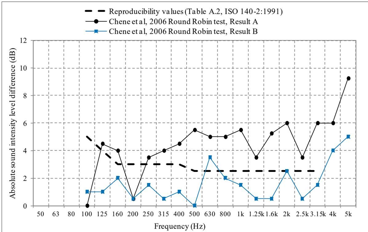
Figure 1 – Interlaboratory variation in measured rain noise levels (Initial)
